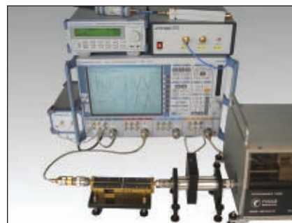
▲ Fig. 10 Setup combining R&S ZVA24 with Focus V-I Probes and MPT multi-harmonic tuner.
