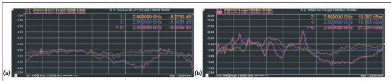
▲ Fig. 5 Measurements of a real SIM-722MH+ mixer, at +10, +13 and +16 dBm LO drive for conversion loss (a) and IP3 (b).
