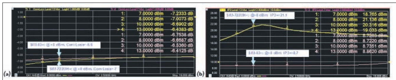
▲ Fig. 6 Conversion loss (a) and IP3 (b) for the SIM-722MH+ and SIM-83+ vs. LO power drive.
