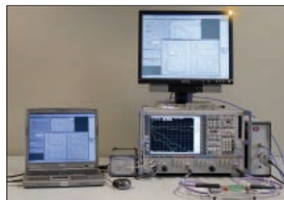
▲ Fig. 3 The NMDG ZVxPlus add-on kit on top of the R&S ZVA24.
